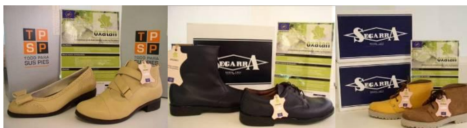
Figure 5. Women's footwear (TPSP), casual and vulcanised footwear (CALZADOS CANÓS GARCÍA, S.L.) manufactured from oxazolidine tanned hides.
