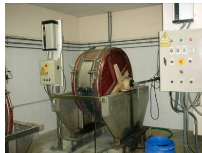
Figure 1. Tanning drum used for bating tests using poultry manure
