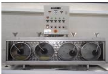
Figures 3 and 4. Laboratory scale and semi-industrial scale fatliquoring tests.
