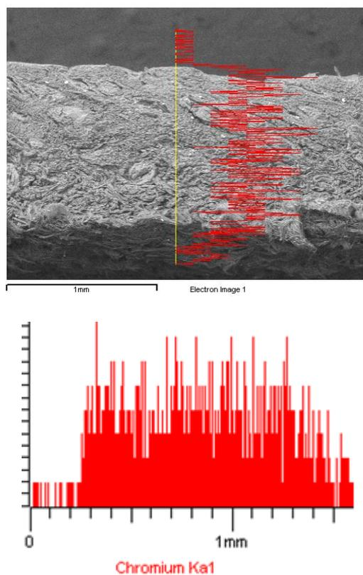
Fig. 1. SEM and SEM-EDX pictures along the section of the traditionally chromium tanned crust leather
