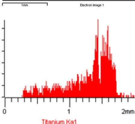
Fig. 2. SEM and SEM-EDX pictures along the section of the innovative titanium tanned crust leather
