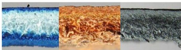
Figure 10. Relationship between anionicity and dye penetration (Syntan 9)
