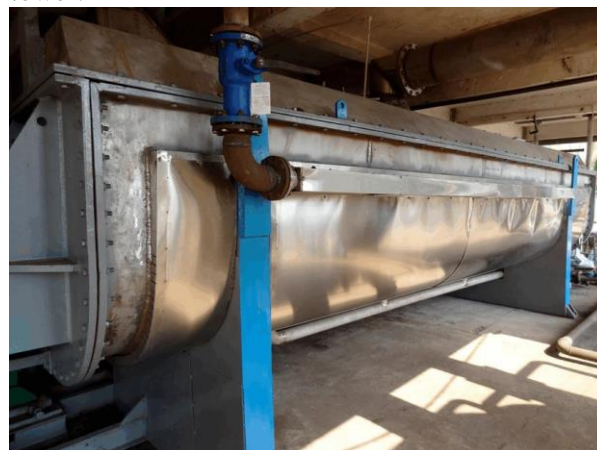
Photo 3: Low cost sludge dryer made in China
