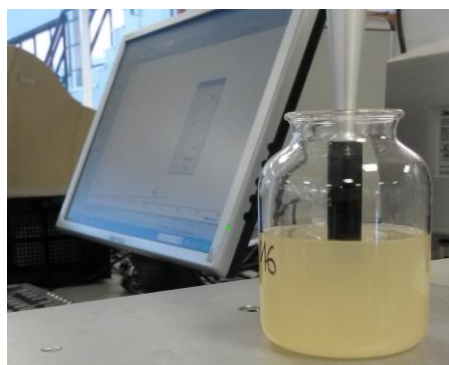
Figure 1. Gel strength (Bloom value) measurement in a texture analyser.
