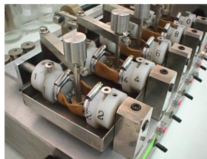
Figure 2. Water resistance test for footwear upper materials according to EN ISO 5403-1.
