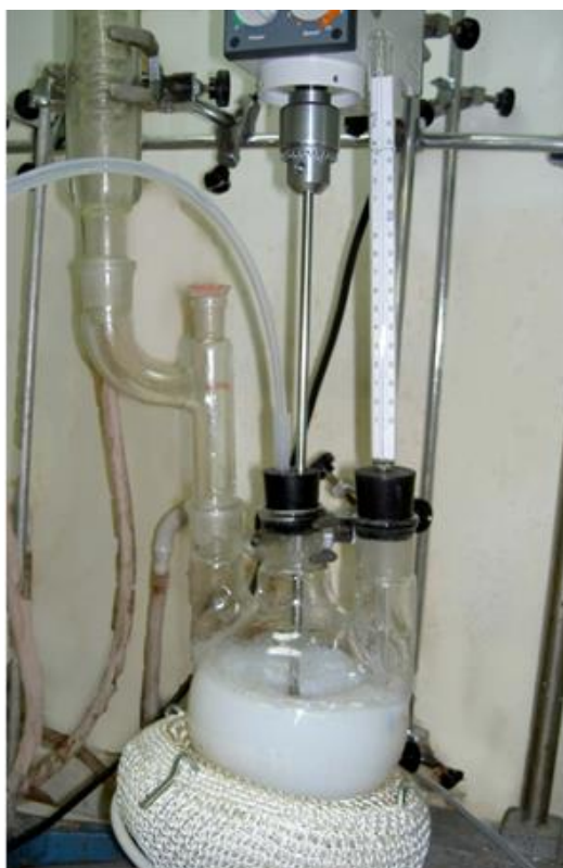
Figure 1. Assembly of the reactor for the resins synthesis
