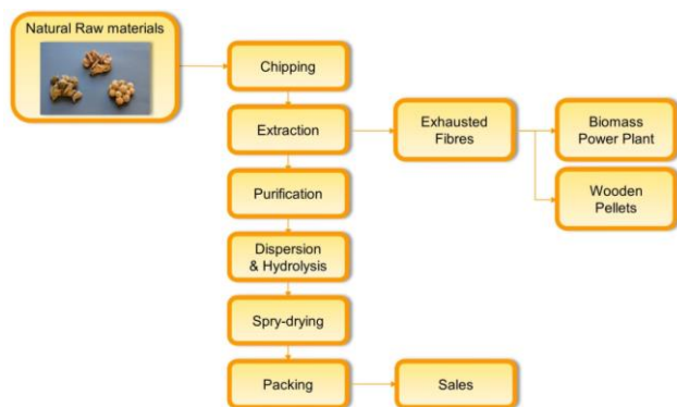
Figure 2 ECOTAN PAP Production Process.
