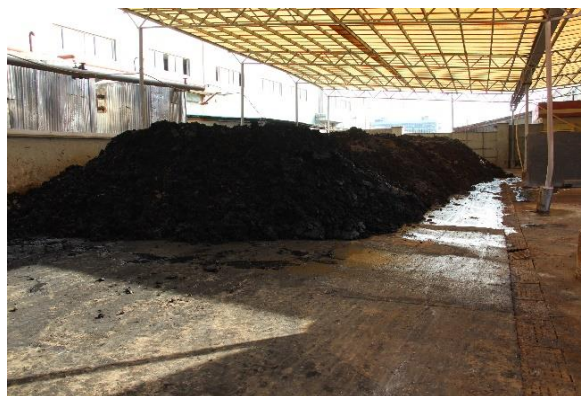
BIOSK technology offers significant reduction in solid waste from effluent treatment for disposal. Recovered hair is chrome free with potential for other uses.
