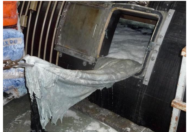
Full release of detritus proteins, fats and salts from within the structure on delimiting and bating.
