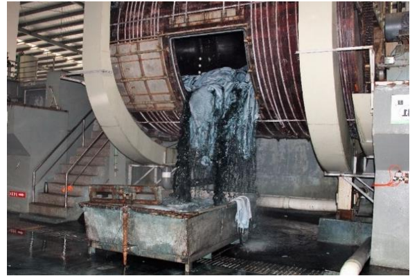
No wash required after chrome tanning as low residual Cr 2 O 3 content in the float. Recovery includes all drainings from stacking areas.
