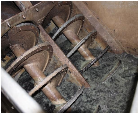
The hair recovery operation. The hair is very intact and serves to filter residual solids and fats from the float.
