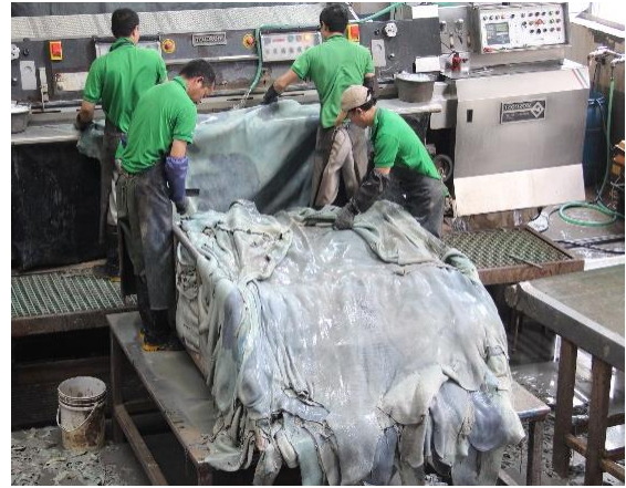
The limed hides from fleshing are clean and relaxed for offer to the lime splitting operation.
