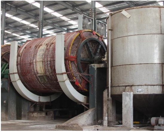
Recovered floats from liming and hair saving processing are held in a single tank fitted with heat exchange systems.
